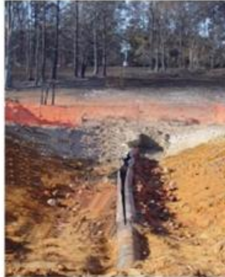
The ruptured pipeline
